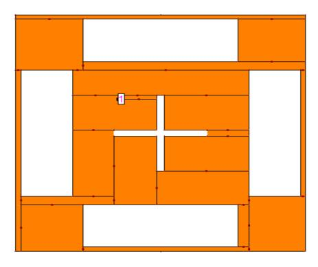
Fig. 1: Geometry of proposed antenna
